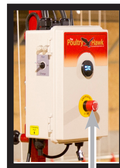
Emergency Stop Button
